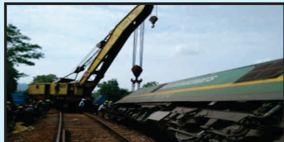
120T CRANE TACKLING TILTED ELECTRICAL LOCOMOTIVE
